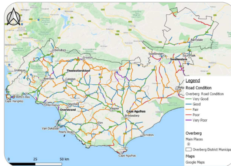
Figure 109: Overberg Road Condition
